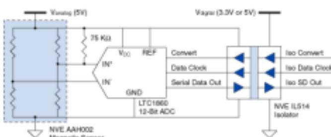
Since the AAH002 is omnipolar (a positive output regardless of field polarity), an inexpensive unipolar ADC is fine. The 75 kilohm resistor ensures the bridge output is always positive, overcoming the bridge's  $\pm 5$  mV/V maximum offset.
