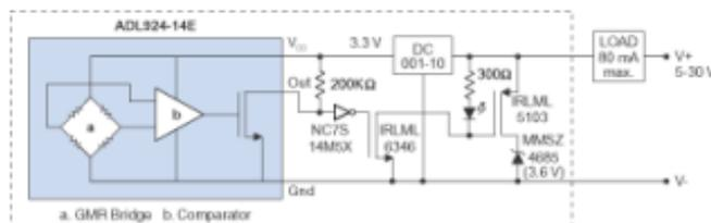
**Two-Wire Reference Circuit Using a Voltage Regulator**
