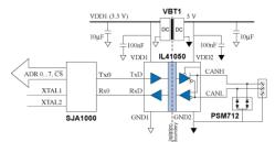
The isolator operates on the 3.3 V microcontroller power supply, and a low-cost dc-dc convertor provides 5 V to power the bus side. The IL41050 can withstand 200 V transients on the bus; the PSM712 provides additional ESD protection if necessary.
